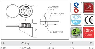
External control gear with 3M cable
