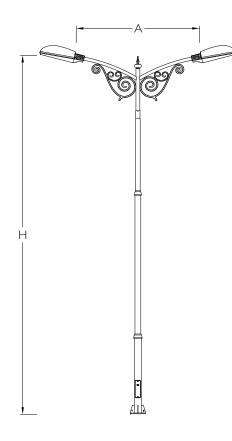
**Finish:** Coated with epoxy zinc phosphate primer and finished using environmentally stable polyurethane based paint.
