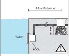
Maximum distance from the fitting to the remote power supply
