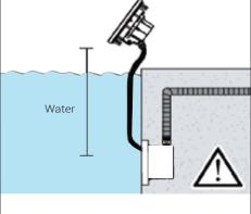
Sufficient cable must be left inside the recess box in order to allow the complete extraction from the water of the fitting for maintenance operation.
